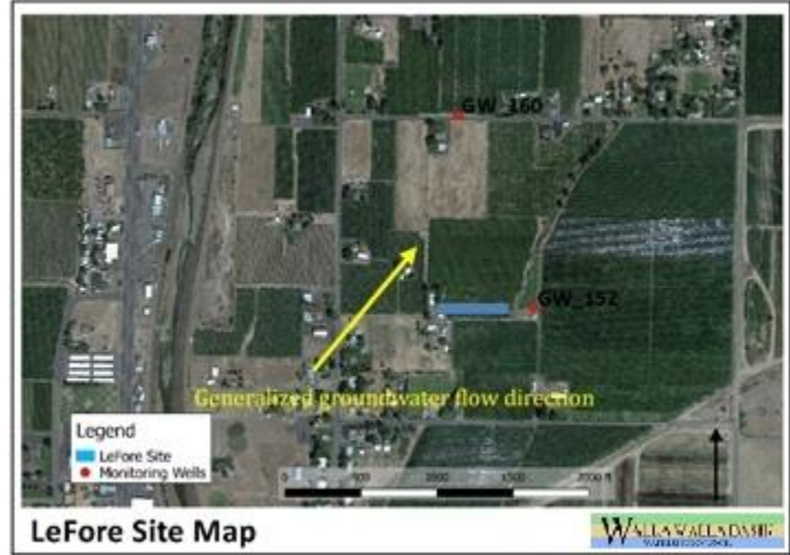
Figure 39. LeFore monitoring well locations.
