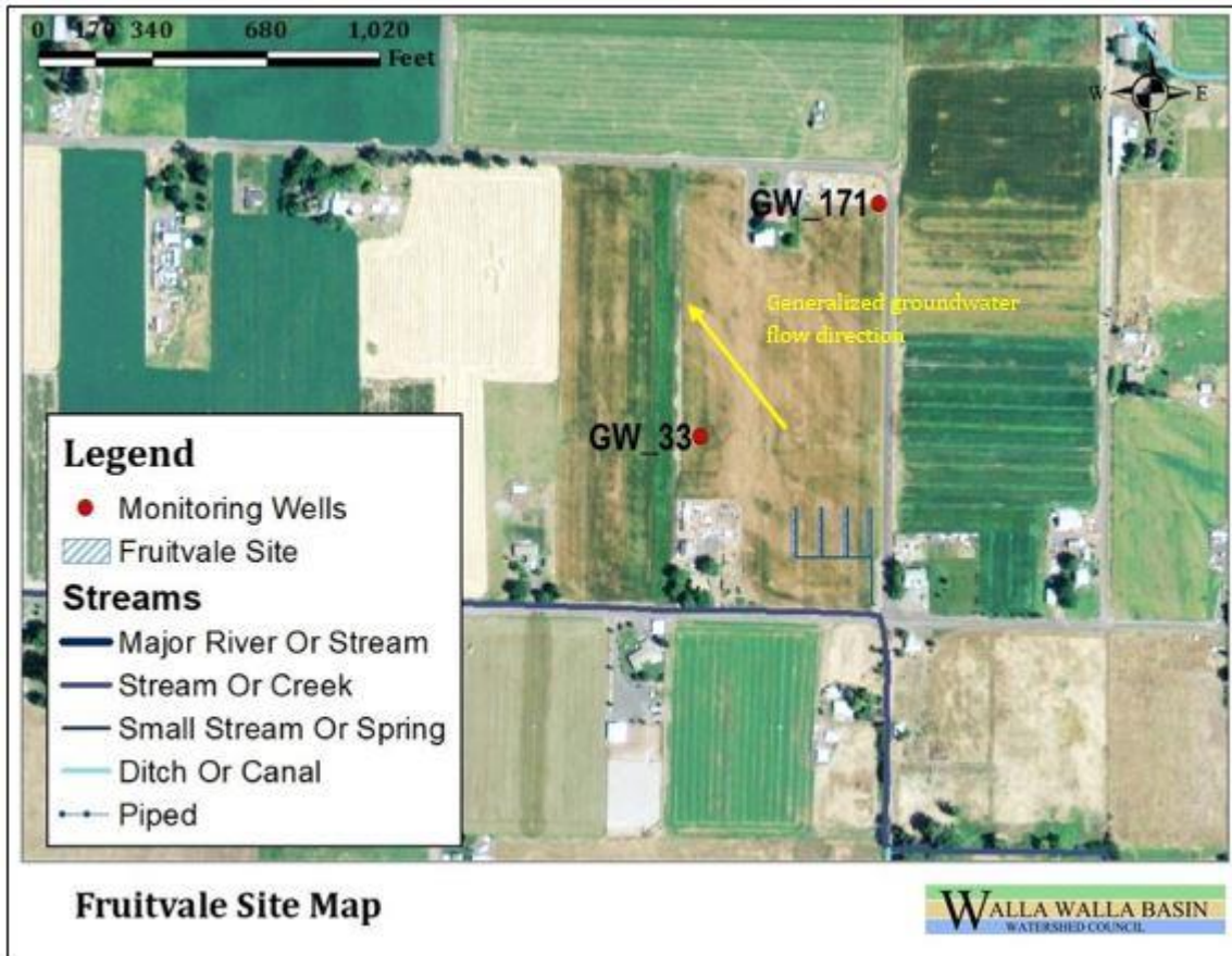
Figure 26. Fruitvale monitoring well locations.
