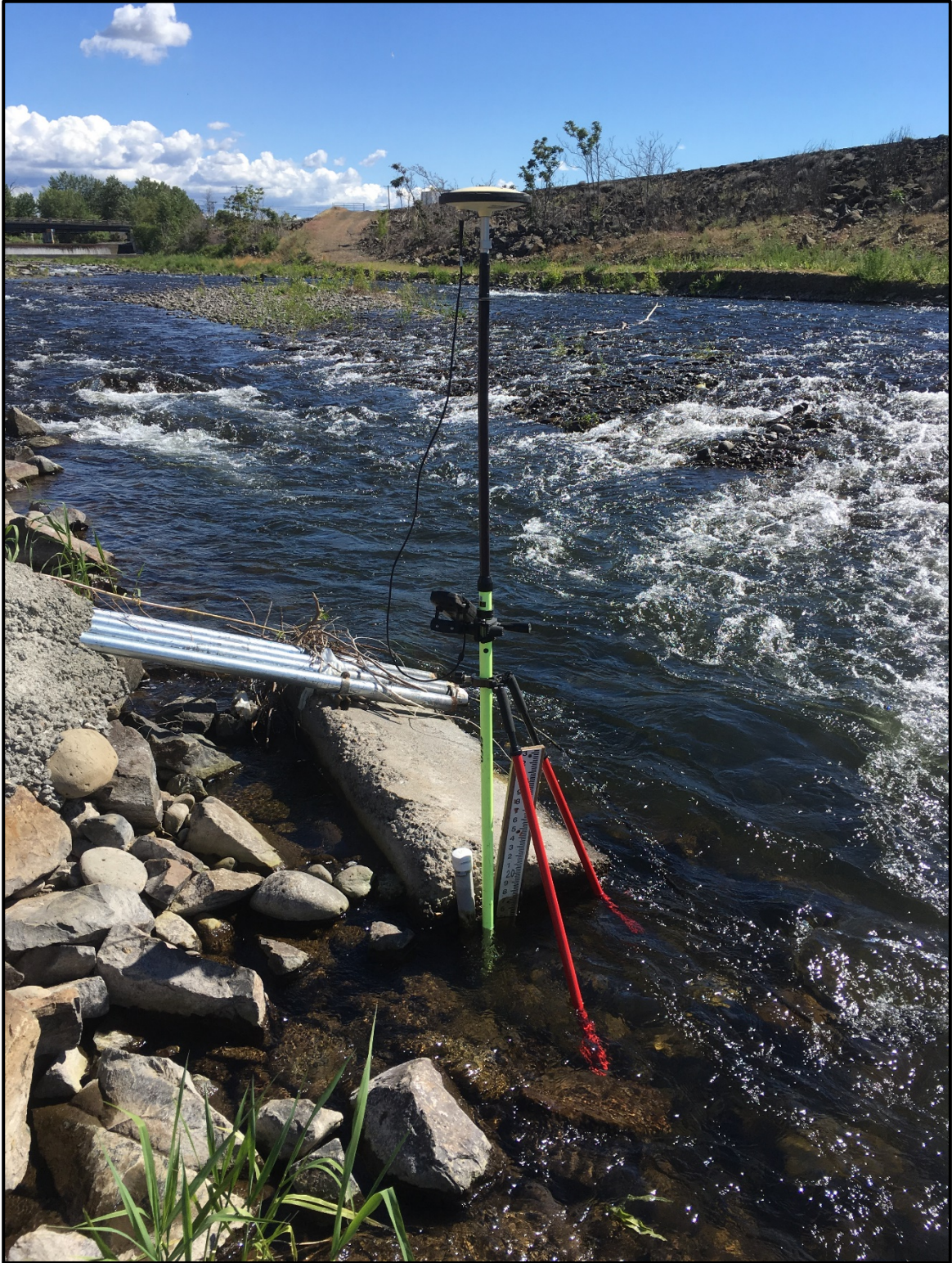
Figure 4. Typical location for GPS measurement at river stage monitoring site. GPS would be placed next to the staff gauge and on the stream/canals substrate. Staff gauge reading and water depth (on survey rod) were also recorded.
