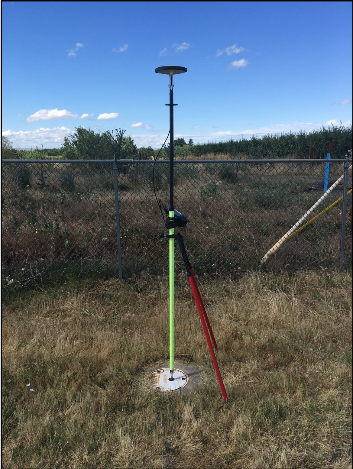
Figure 2. Typical location for GPS measurement at purpose built groundwater monitoring locations.
