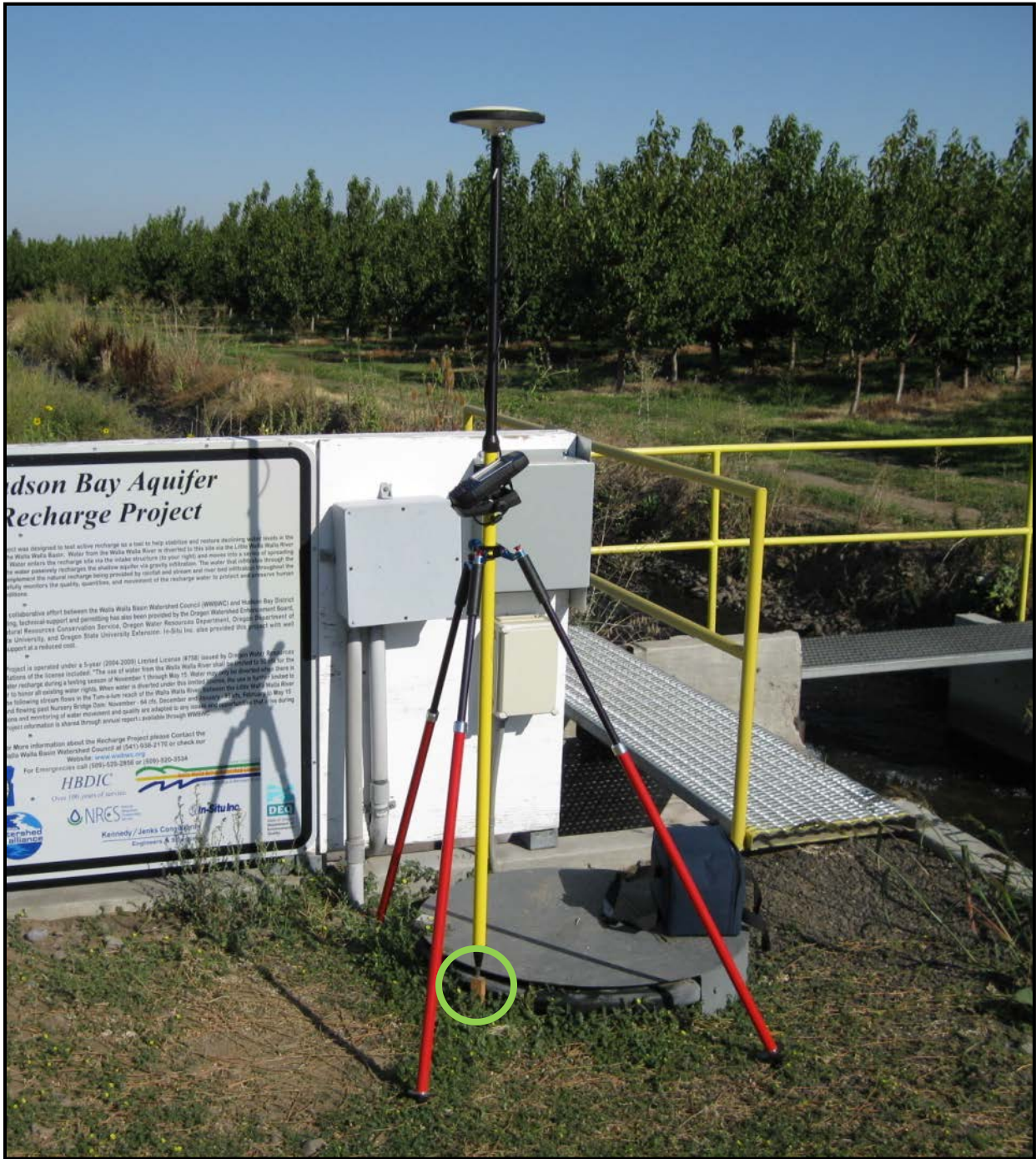
Figure 1. BASE unit located at HBDIC Aquifer Recharge Project site. Notice the bottom of the BASE unit is on a stake with a screw (green circle) for accuracy when repeatedly setting up the BASE unit.
