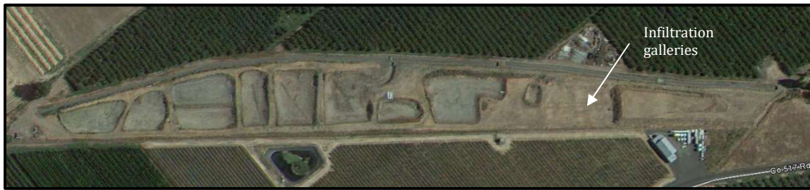
Figure 17. Johnson site in 2013 showing 10 basins and location of infiltration galleries.
