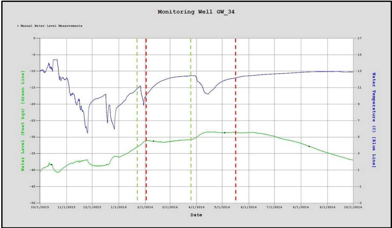
Figure 45 - Hydrograph for monitoring well GW_34. Green dashed lines indicate start of recharge operations and red dashed lines indicate end of recharge operations.
